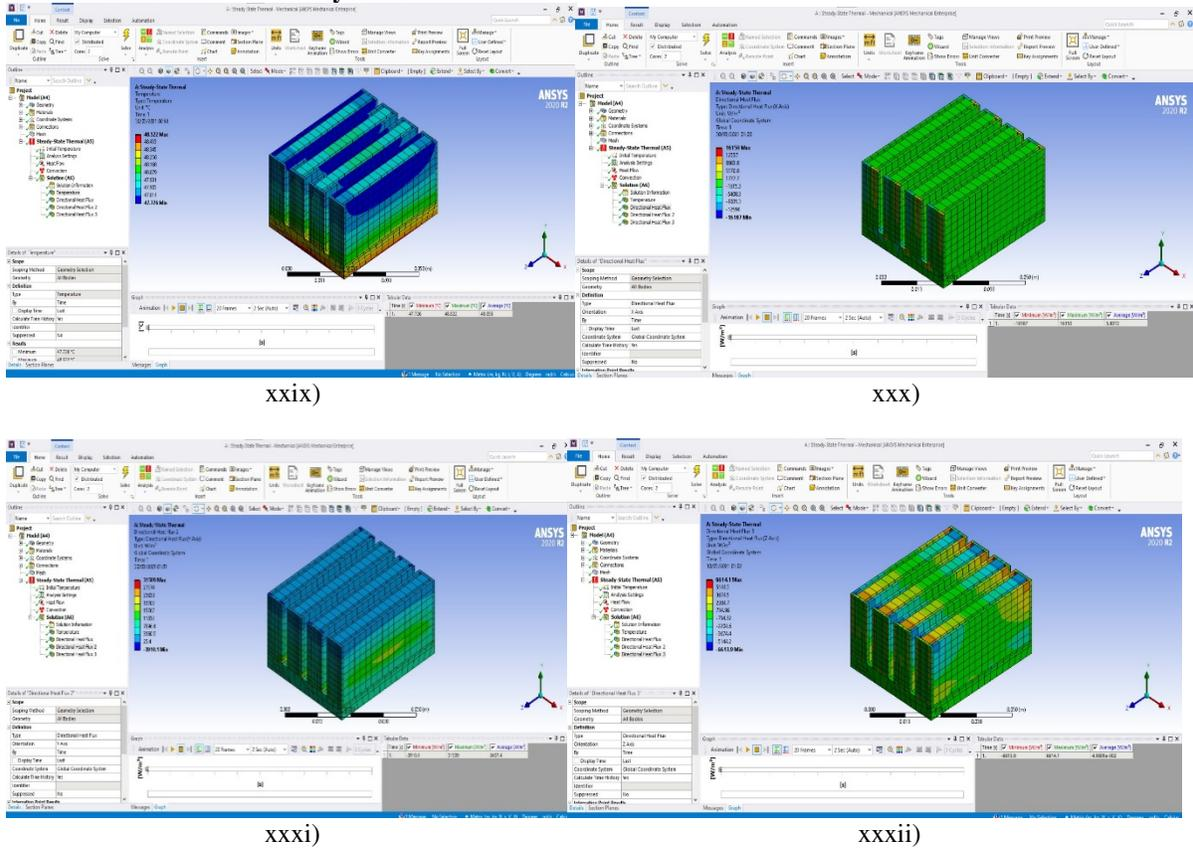
**Figure 15:-Steady state thermal analysis of inverted-T non-perforated fin using Ansys®.**
