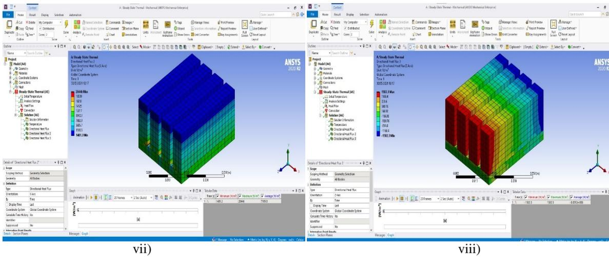
Figure 9:- Steady state thermal analysis of rectangular non-perforated fin using Ansys®.
