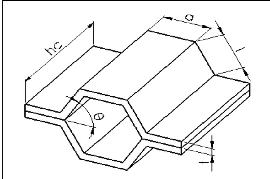
Figure 3:- 3D view of the perforated honeycomb.
