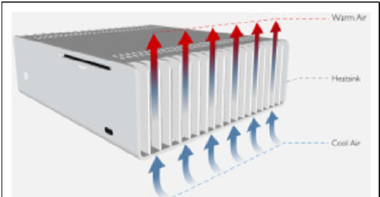
**Figure 1:-** Principle of Heat Sink (20).
