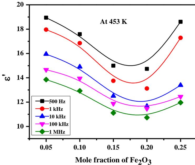
**Figure 5:-** Compositional dependence of dielectric constant,  $\epsilon'$ , for the BFN glasses at 453 K and for different frequencies. Solid lines drawn are guides to the eye.
