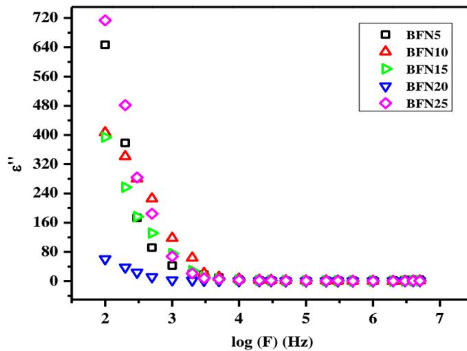
Figure. 3:- Plot of log(F) versus ( $\epsilon''$ ) at T=453K temperature for all glasses.
