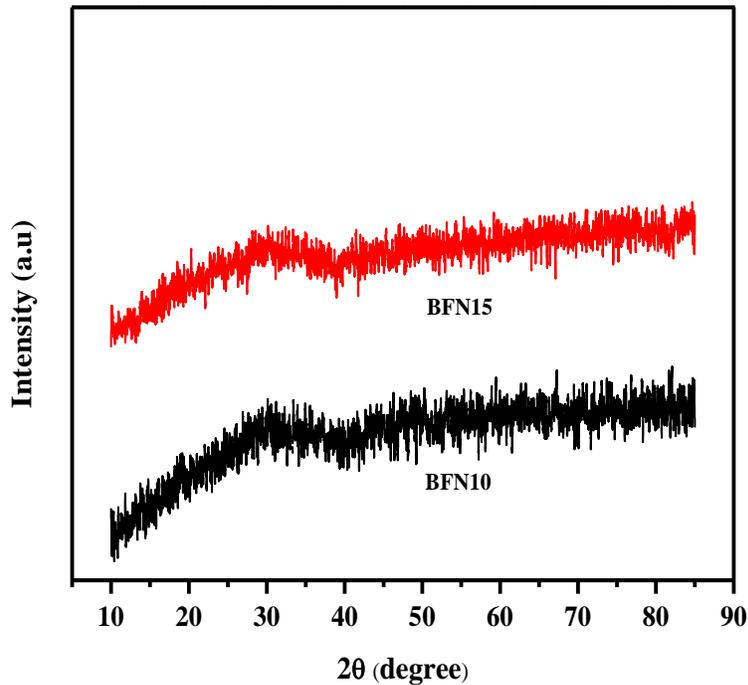
**Figure 1:-** X-ray diffraction pattern of BFN10 and BFN15 samples.
