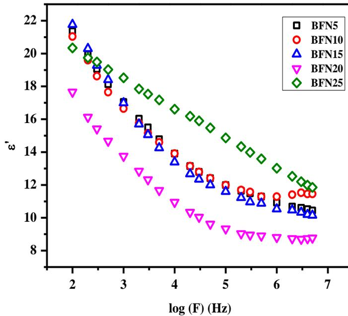
Figure 2:- Plot of log (F) versus ( $\epsilon'$ ) at T=453K temperature for all glasses.
