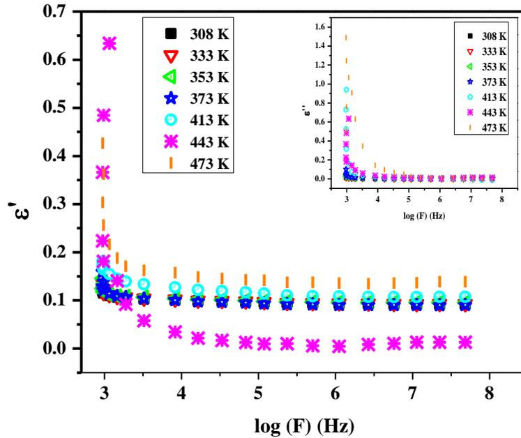
**Figure 4:-** Plot of  $\log(F)$  versus  $(\epsilon'')$  for the glass BFN20 at different temperatures. Inset shows the frequency dependency of  $\epsilon''$  for the glass sample BFN20.
