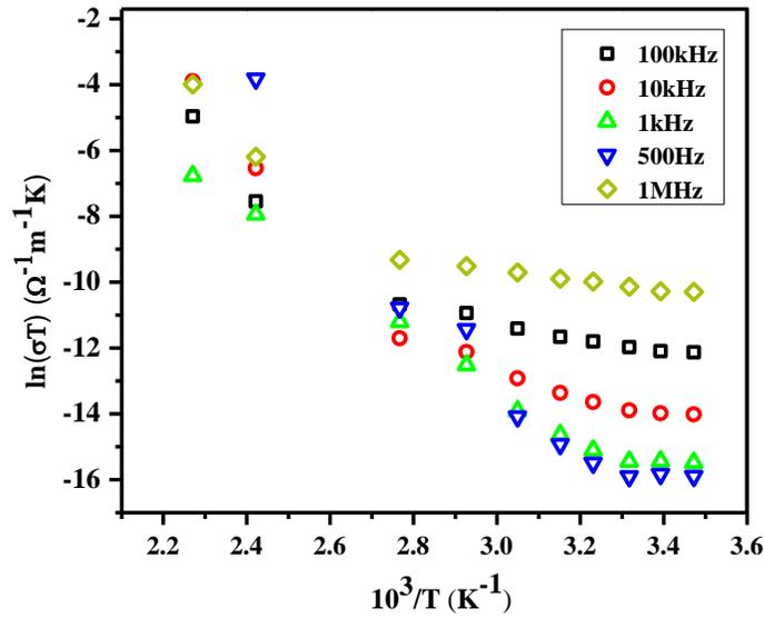
Figure 7:- Temperature dependence of ac conductivity at different frequencies for the glass BFN20.
