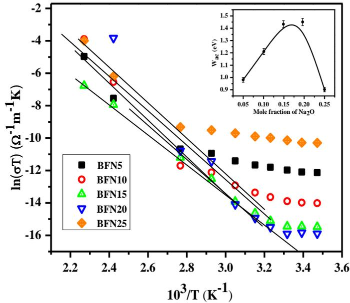
**Figure 6:-** Temperature dependence of ac conductivity at 100 kHz for BFN glasses. Solids lines are the least square linear fits to the high temperature data. Inset shows the variation of ac activation energy with composition.
