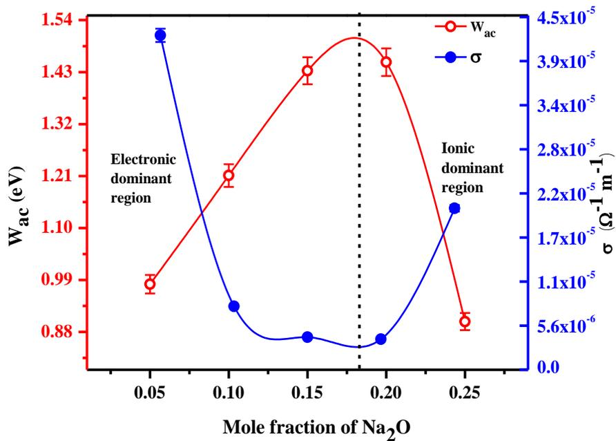
Figure 8:- Compositional variation of activation energy,  $W_{ac}$ , and conductivity at 453K and at 100 kHz for the BFN glasses. The lines are drawn as guide to eye.
