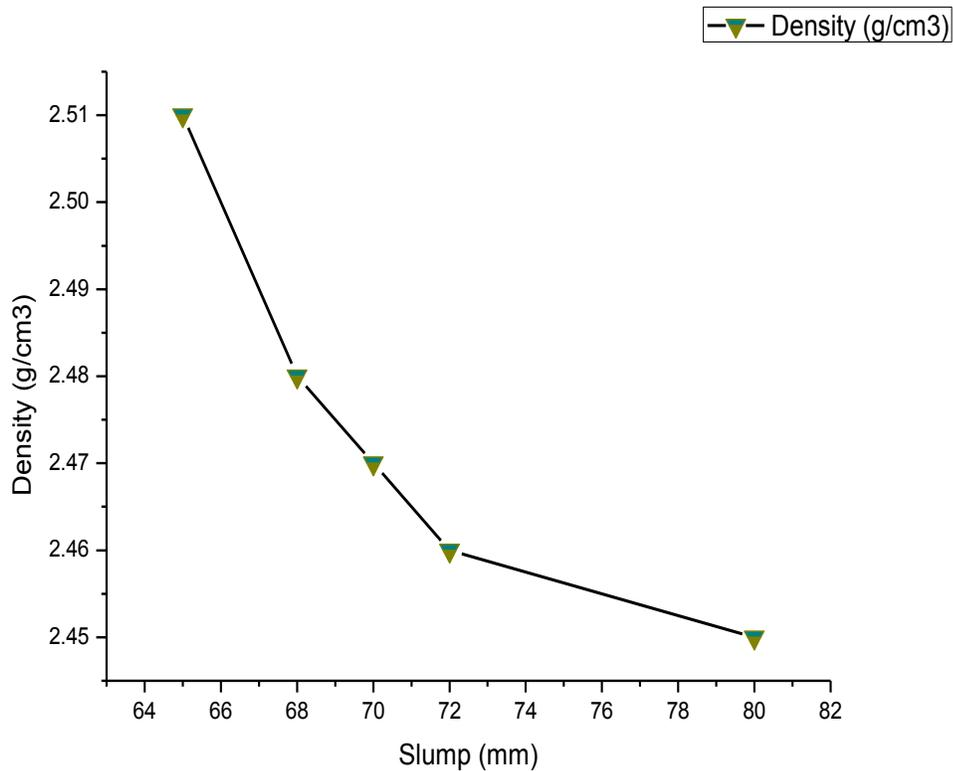
**Figure 4:-** Workability as a function of the density of the mixes.
