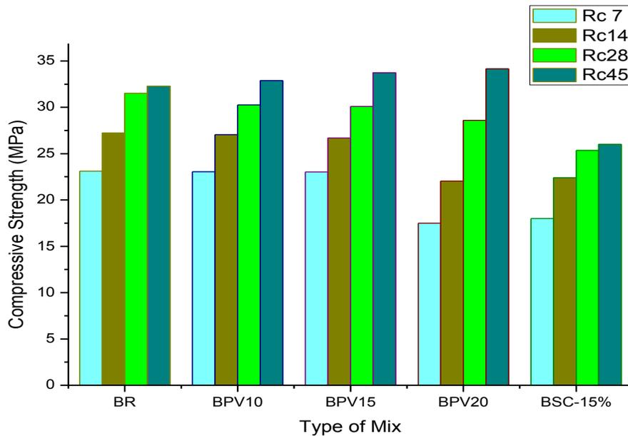
Figure 7:- Compressive strength at 7, 14, 28 and 45 days age.
