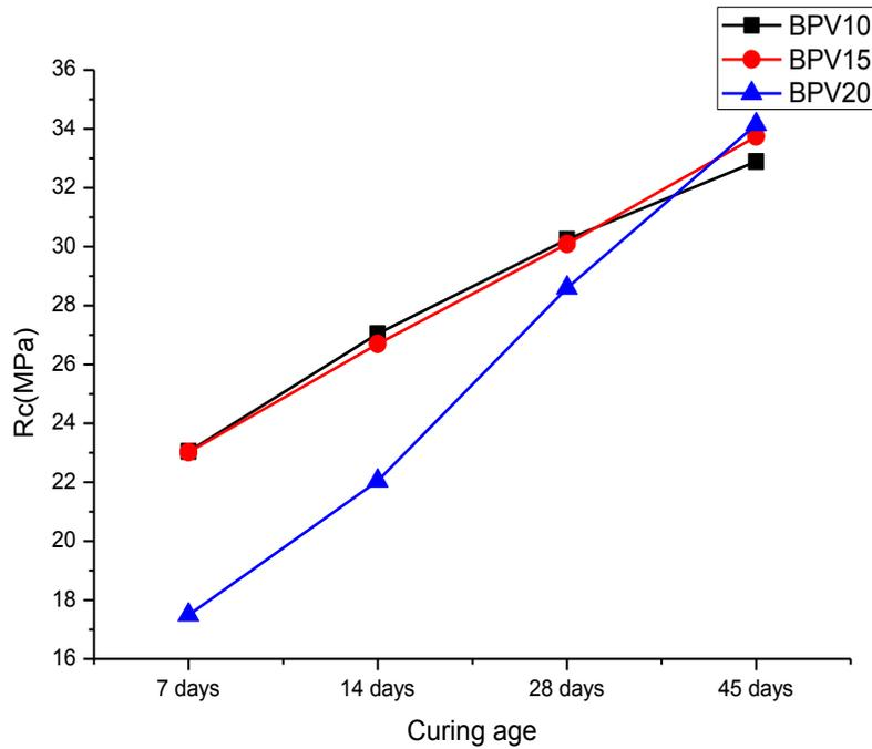
**Figure 8:-** Compressive strength development over time with Glass Powder.
