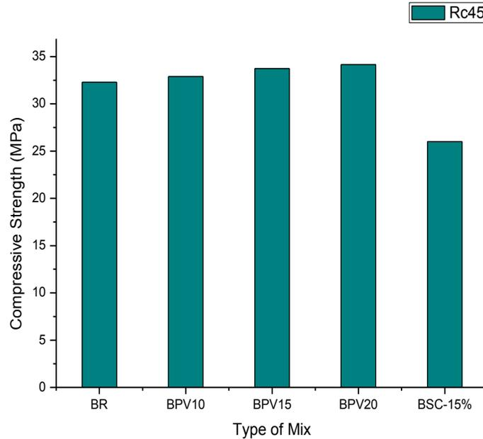
Figure 6:- Compressive Strength at 45 days.
