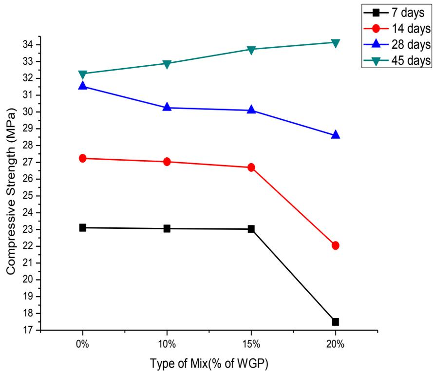
**Figure 9:-** Compressive strength as a function of the content of Glass Powder.
