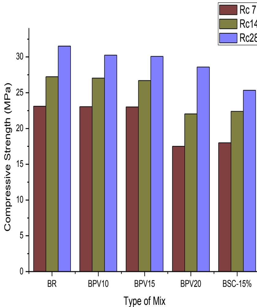
**Figure 5:-** Compressive Strength at 7days, 14 days and 28days.
