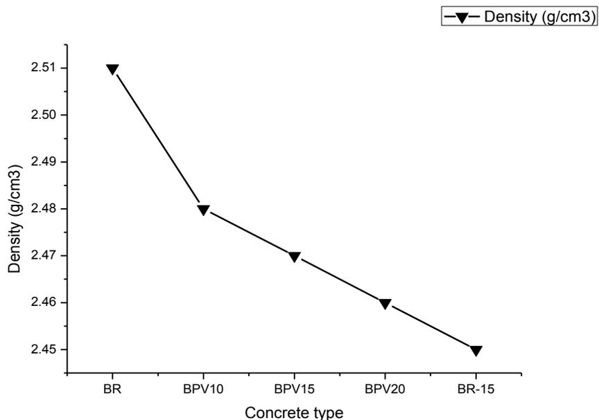
Figure 3:- Density of the concrete specimen.
