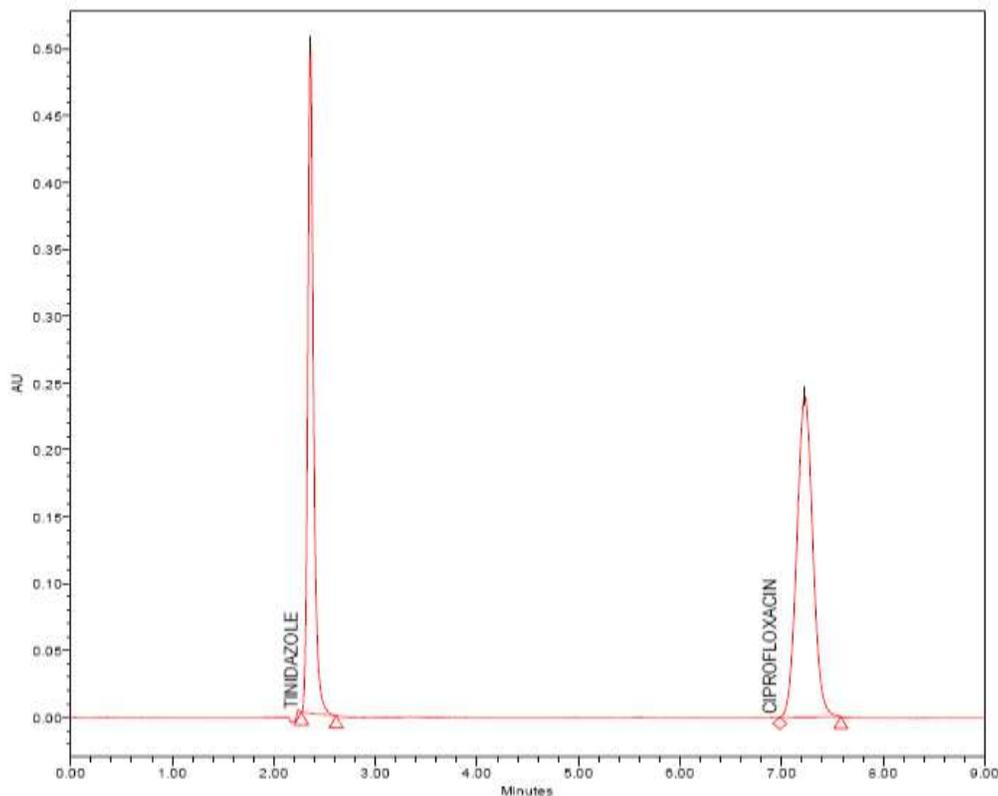
**Figure 2:-** Typical Chromatogram of standard Tinidazole and Ciprofloxacin.
