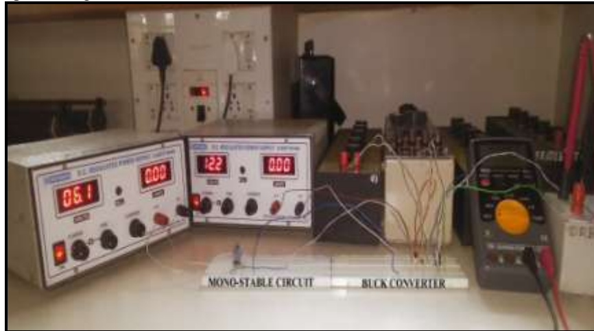
Fig 9:- MOSFET triggering with Mono-stable multi-vibrator
