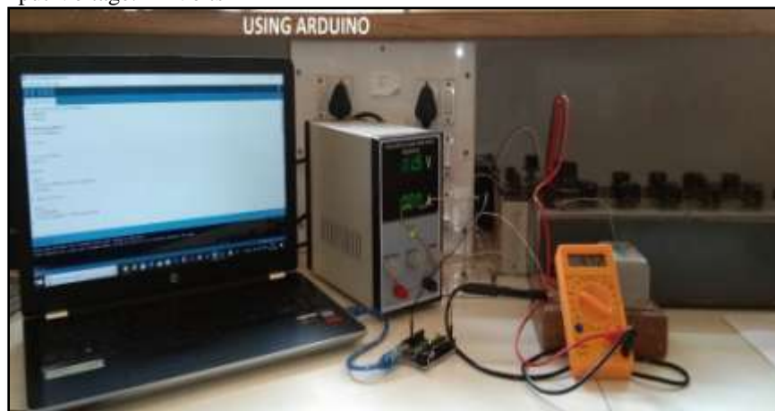
Fig 10:- MOSFET triggering with Arduino with feedback system.
