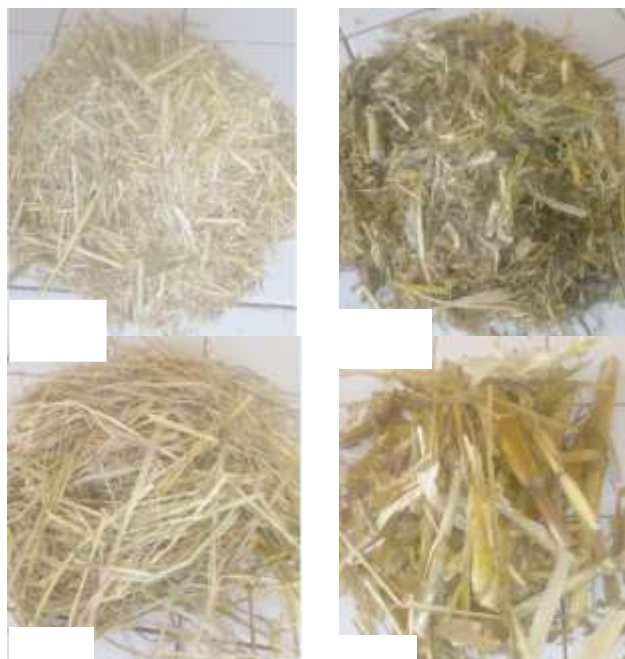
Figure 6:- Products from the mechanical grinding of rice straw (a) and corn (b) and manual grinding of rice (c) and corn (d)
