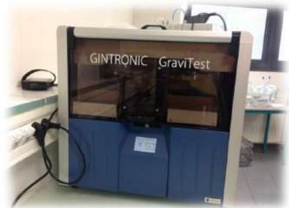
Figure 5:- Experimental device for measuring water vapour permeability by the GintronicGravitest cup method [1].
