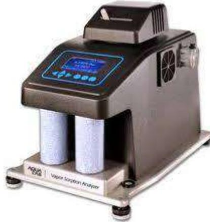
**Figure 2:-** Device for measuring isotherms according to the VSA (Vapour Sorption Analyzer) (DECAGON-Aqualab-USA) [1].
