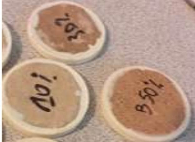
**Figure 14:-** Samples used for the water vapour permeability test
