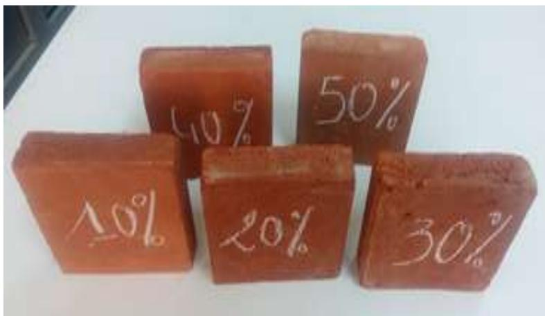
**Figure 10:-** Earth specimens for thermal tests.
