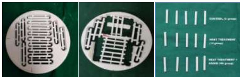
Fig. 4 Fig. 5 Fig. 6 Fig. 4& 5:- ( milling), Fig. 6(15 samples of size 28mm×4mm×2mm)
