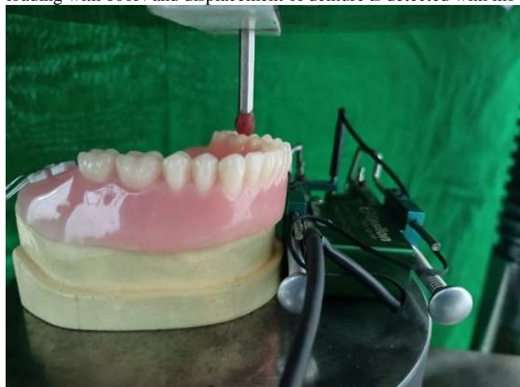
Fig:7:- Molar loading with 100N and displacement of denture is detected with movement sensor
