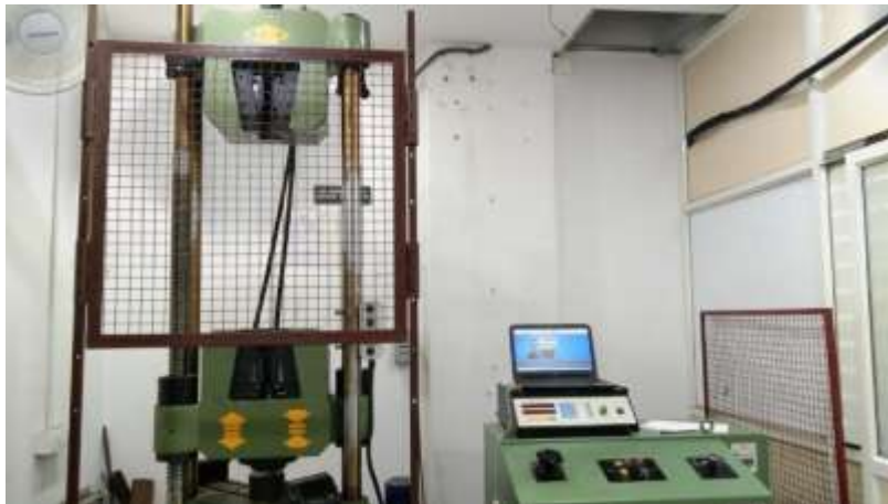
Fig. 5:- Universal testing machine.
