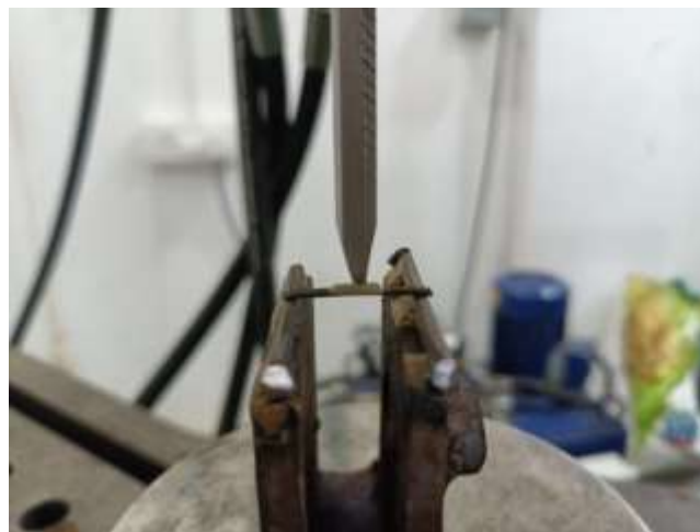
Fig. 6:- 3 point bend test.
