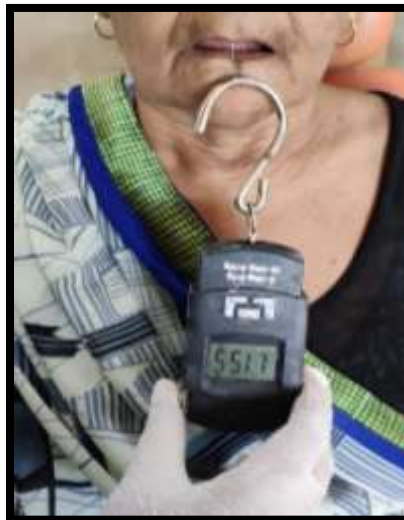
Fig 3:- Digital force gauge was used to measure the retention.
