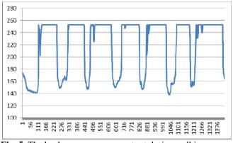
Fig. 5. The heel pressure sensor output during walking.
