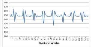
Fig. 4. The Z acceleration during walking.
