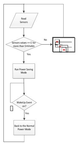
Fig. 3. The Power module flow diagram.
