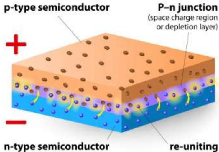
**Figure 1:-** P-N junction semiconductor.
