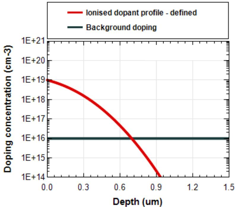
Figure 3:- Doping concentration for silicon with boron doped background versus the junction depth.
