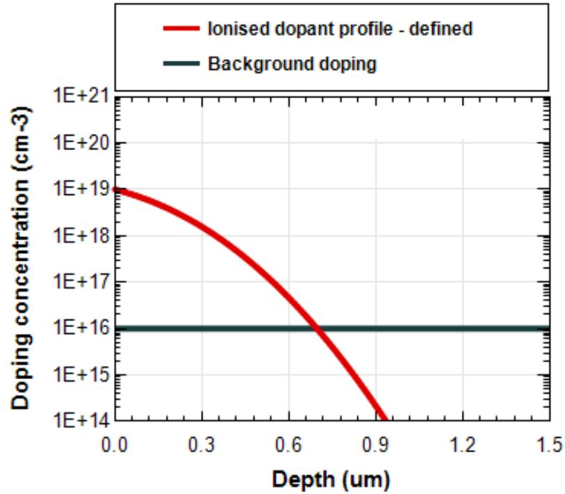
Figure 2:- Doping concentration for silicon with boron doped background versus the junction depth.
