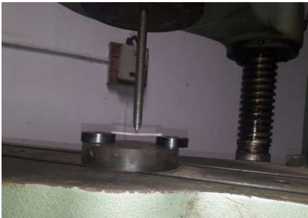
Figure 12:- Load applied in repaired area of the specimen.
