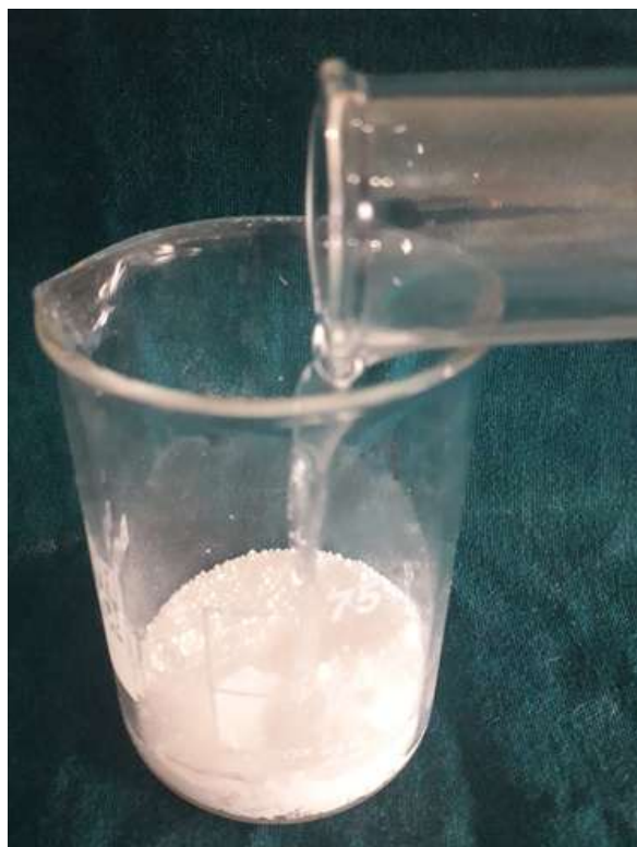
Figure 9:- Addition of acetone into nanoparticles.
