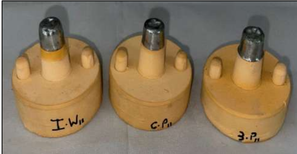
Fig. 5:- Group A, Group B and Group C coping trial on die.
