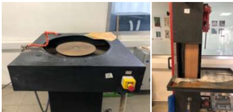
Figure 19:- Sanding Machines to Make the Glass Sharp Edges Smooth, ARUCAD Glass Studio, 2023.
