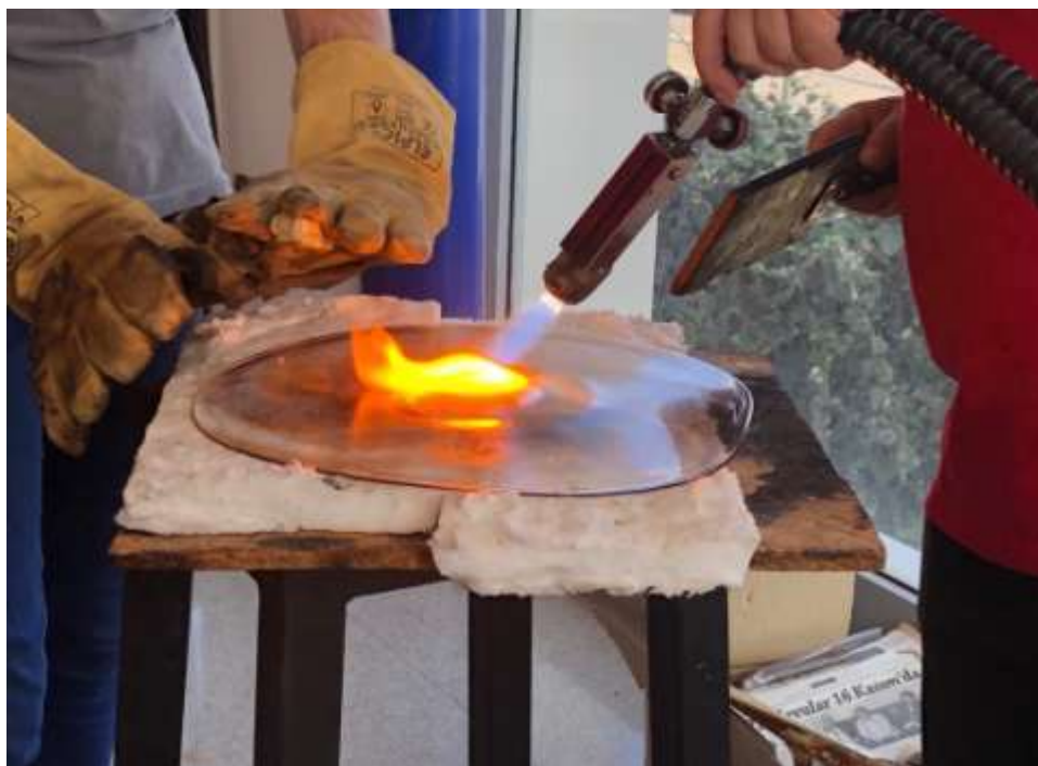
Figure 16:- Sevda Orr, the use of torch, and wooden paddle to smooth the surface of the area of where the glass was detached from punty, 2022.
