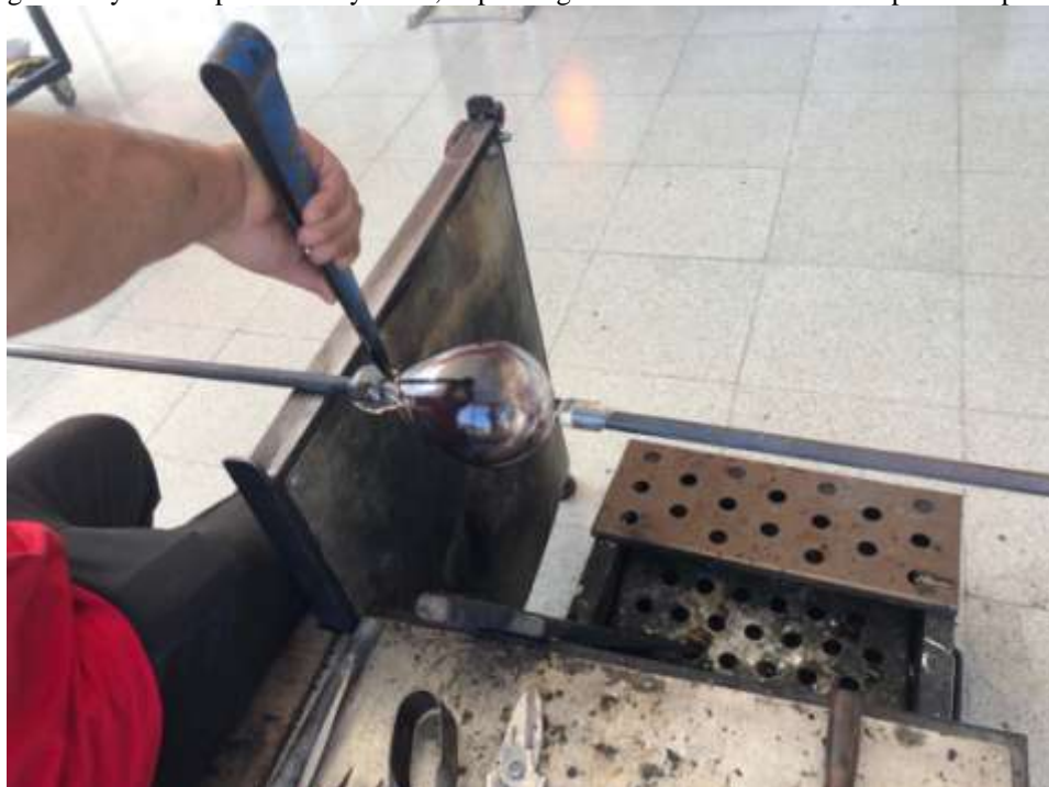
Figure 12:- Attaching the punty to the bottom of the piece with a molten glass, the one on the pipe on left is the punty, glass studio, 2022.
