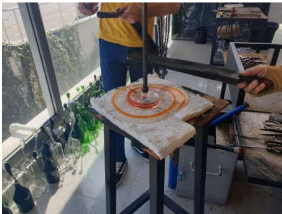
Figure 15:- The glass piece was put on the heat resistant blanket to detach from punty, glass studio, 2022.
