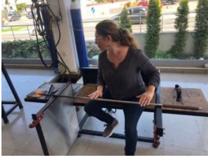
Figure 8:- the bench, blowpipe with molten glass and sitting of the glass blower, Glass Studio, 2023
