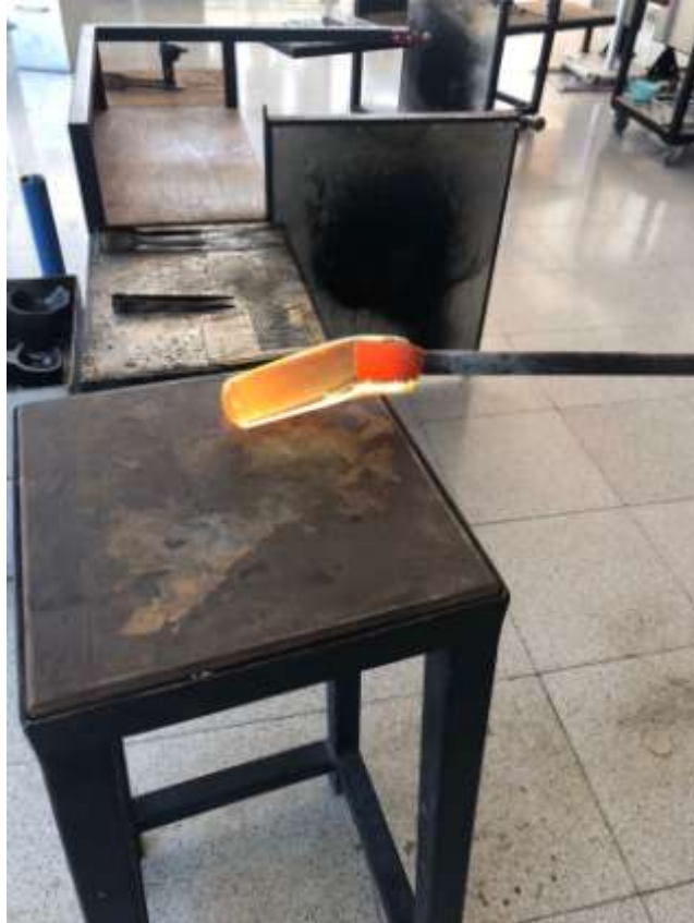
Figure 4, Shaping the first take of molten glass on the surface of the marver, ARUCAD glass studio, 2022
