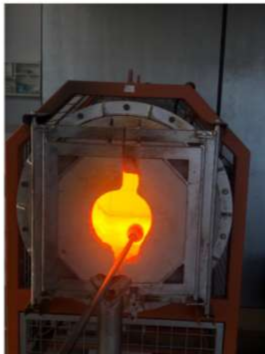
Figure 5:- The mouth of the furnace is called "glory hall", the blowpipe is resting on the yoke, ARUCAD glass studio, 2022.
