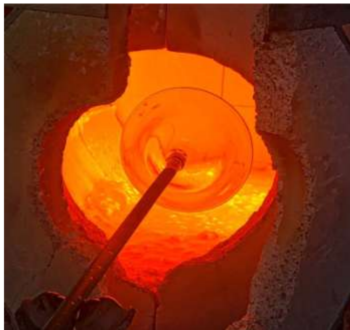
Figure 14:- The glass piece is formed and then put it the furnace to make it malleable, 2022.
