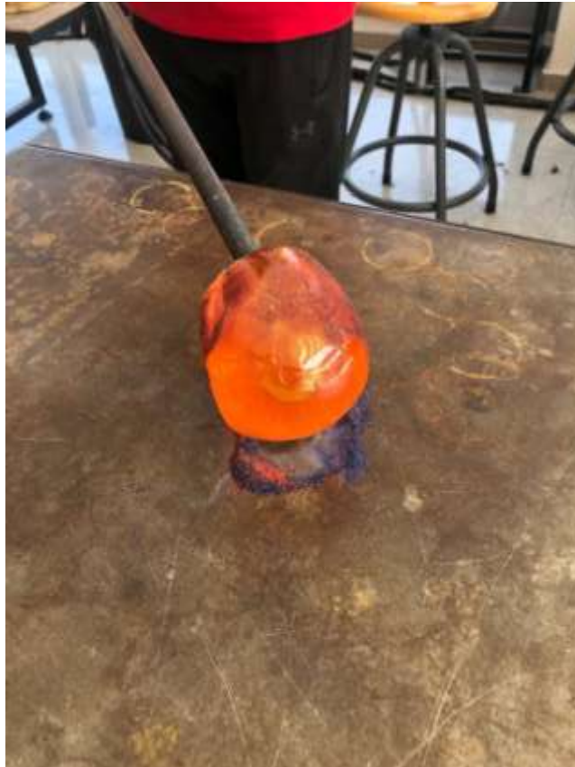
Figure 11:- Getting colour onto the molten glass from the marver, glass studio, 2022.
