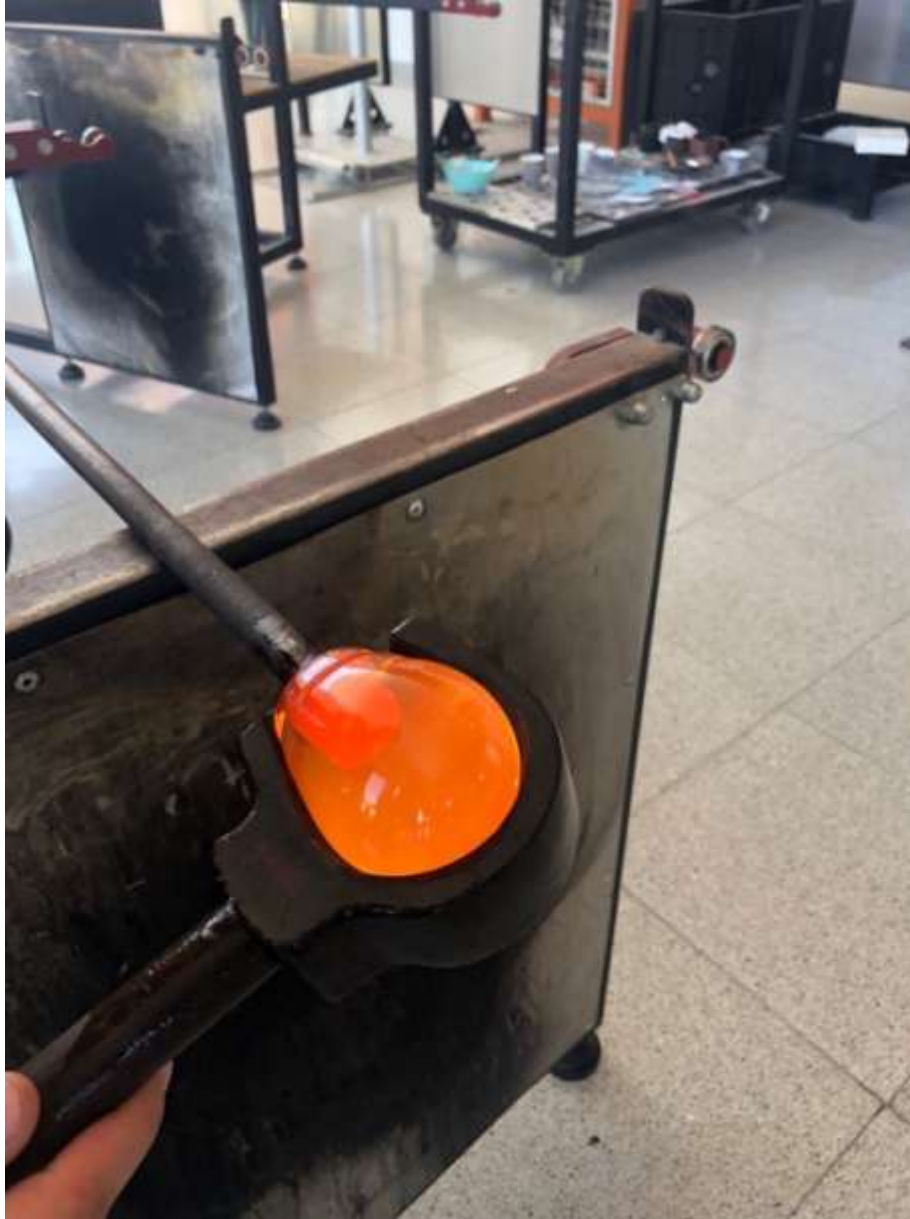
Figure 7:- Shaping the molten glass with block, ARUCAD glass studio. 2023.
