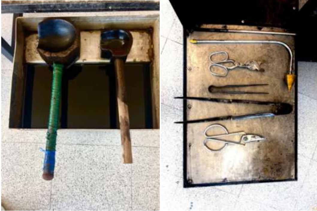
Figure 2:- On the left big and small blocks (wooden spoons); on the right; sophietta, diamond scissors, small and big jacks and shears.
