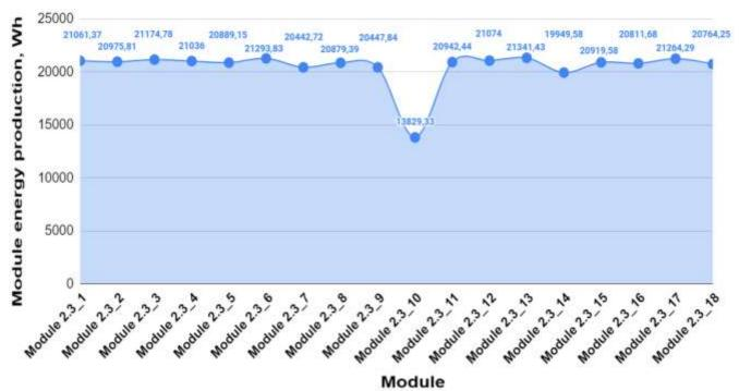
Figure 3:- Energy generated by the solar panels of the chain with the number String 2.3.
