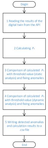
Figure 5:- Block diagram of the software algorithm for finding anomalies in the operation of solar panels, developed on the basis of the proposed methodology.
