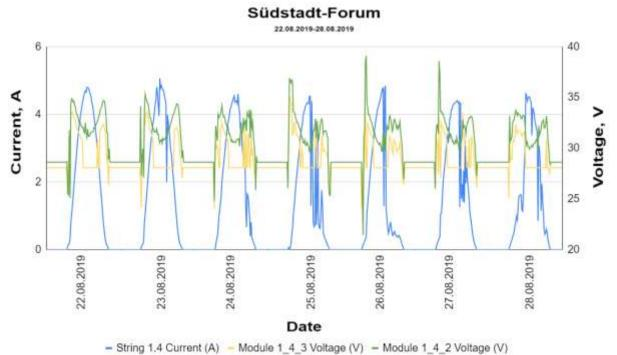
Figure 1:- Curves of voltage and current of solar panels with numbers Module 1.4\_2 and Module 1.4\_3.
