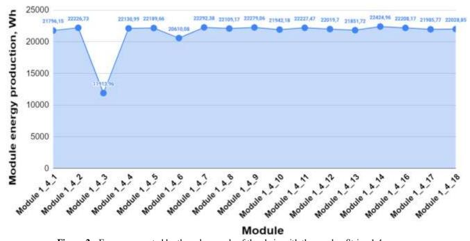
Figure 2:- Energy generated by the solar panels of the chain with the number String 1.4.
