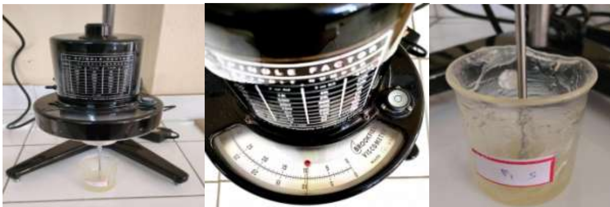
Fig 1,2 and 3:- Brookfield Viscometer for Rheological determination of Kinetic Viscosity.
