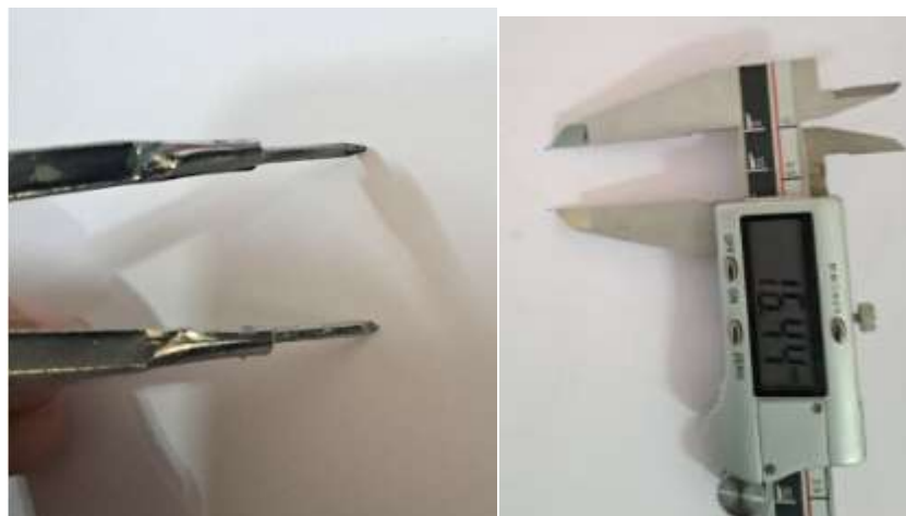
Fig. 5:- Marks transferred to white paper by divider and measured with the help of digital verniercaliper.
