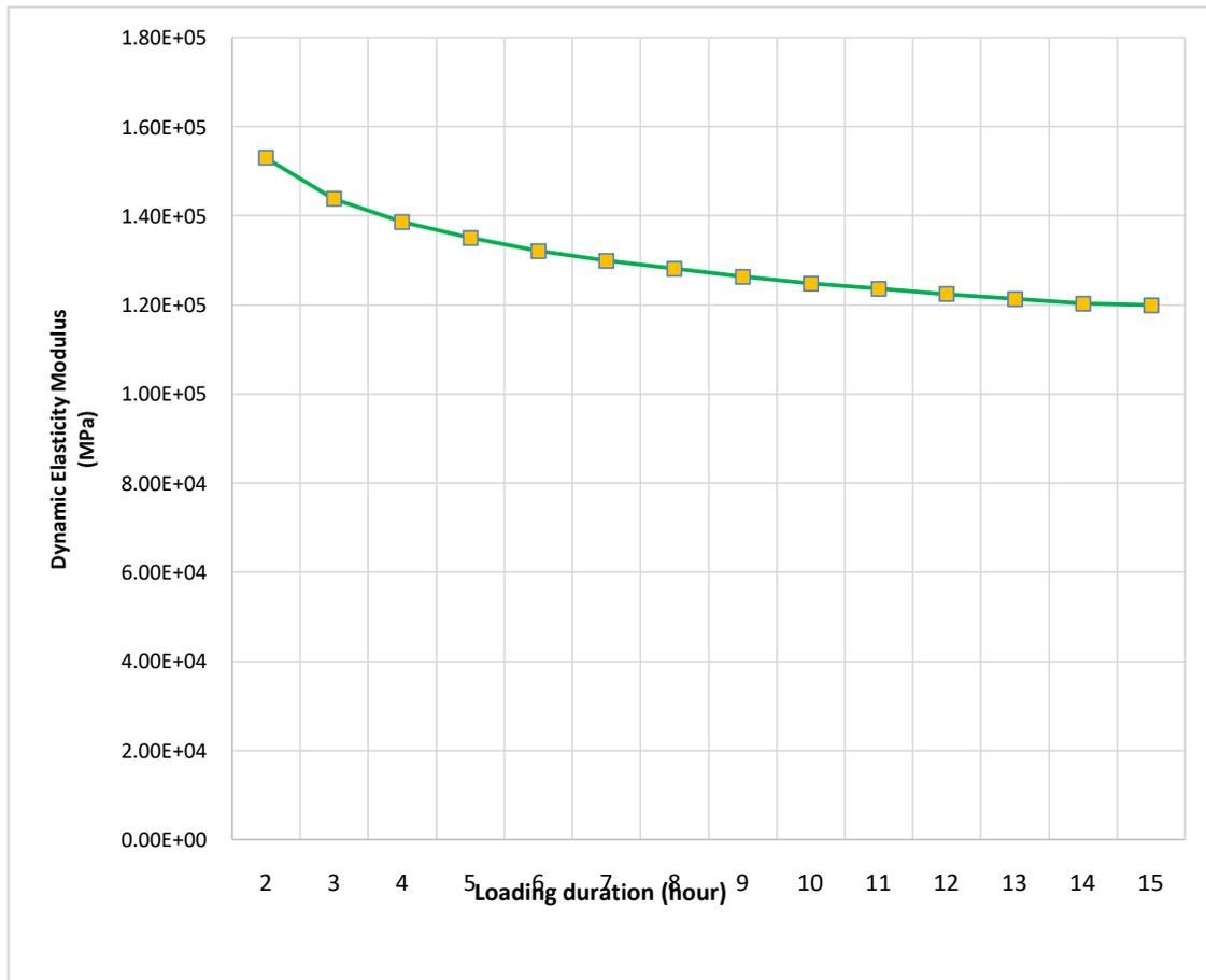
Fig. 4:- Evolution of the dynamic elasticity modulus as a function of loading duration.
