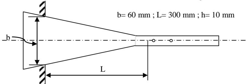
Fig. 2:- Experimental device for bending creep test.
