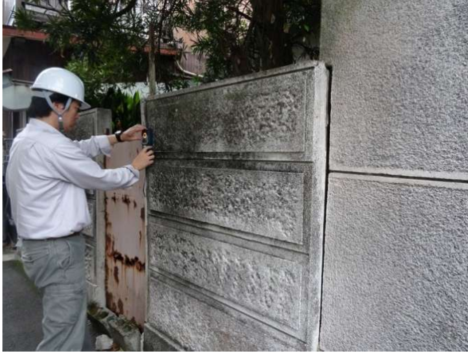
Fig 6:- Investigation of presence or absence of rebars using sensors.
