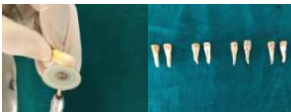
Figure 8a & 8b:- (8a) Polishing the Bond Interface using 400 & (8b) 1000 Grit Abrasive Paper.
