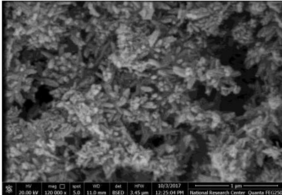
**Figure (3a):-** SEM micrograph of the prepared hydroxyapatite nanoparticles.
