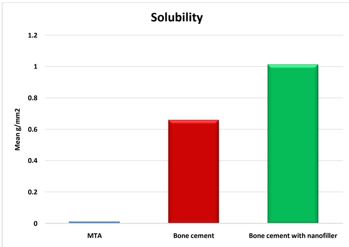
**Figure (5):-** Bar chart showing mean values of solubility results of MTA, bone cement and bone cement with calcium hydroxyapatite nano filler.
