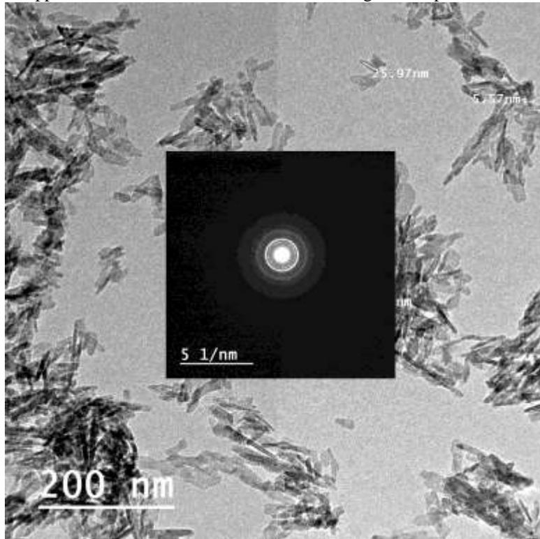
**Figure (4):-** TEM micrograph of the prepared hydroxyapatite nanoparticles.
