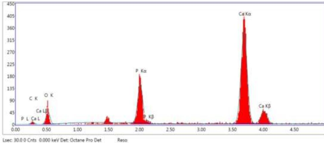
**Figure (3b):-** EDAX analysis of the prepared hydroxyapatite nanoparticles.
