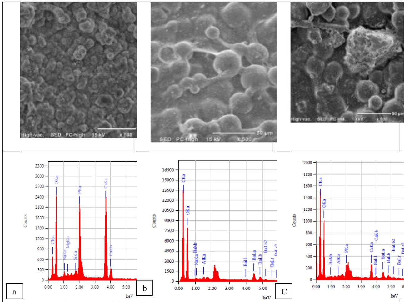
**Figure (5):-** SEM micrographs and EDX analysis of the tested groups after immersion in SBF for 21 days : a) MTA sample (x500) b) PMMA bone cement sample and c) PMMA composite sample.
