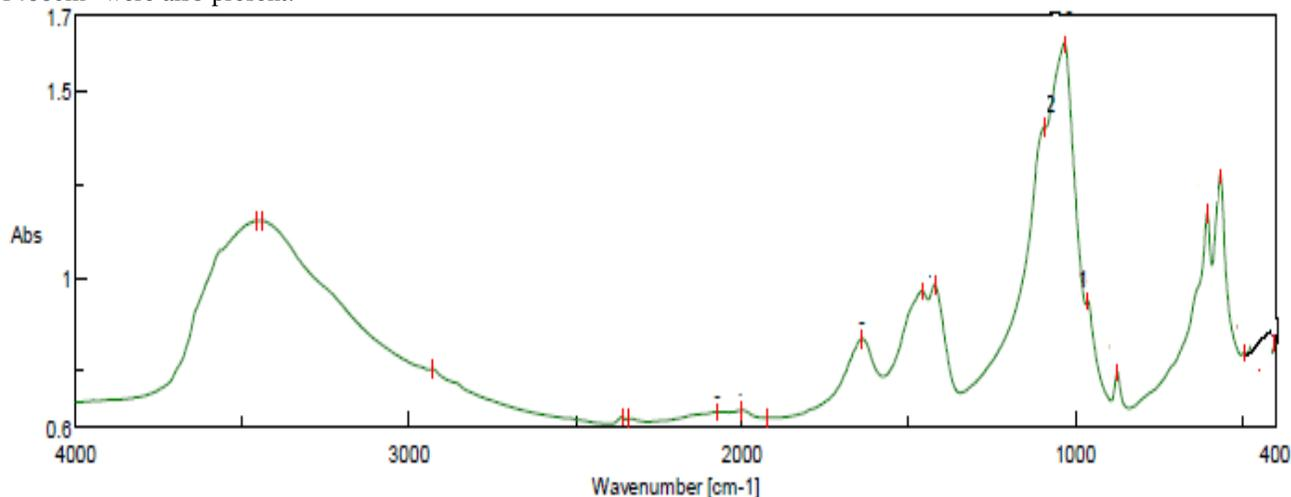
Figure (1):- FTIR analysis of the prepared hydroxyapatite nanoparticles.
