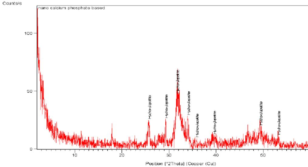
**Figure (2):-** XRD analysis pattern of the prepared hydroxyapatite nanoparticles.
