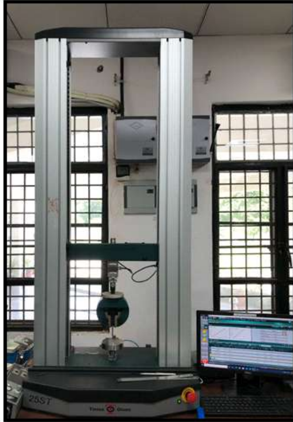
Fig 1:- Universal instron testing machine.
