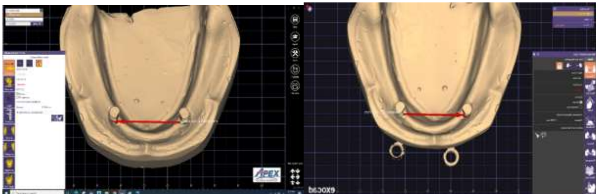
Fig (6 a & b):- Distance between the two implant analogs measured from the same reference pint by Software's of DofFreedom X5 premium and Medit T300-T500 dental lab scanners.
