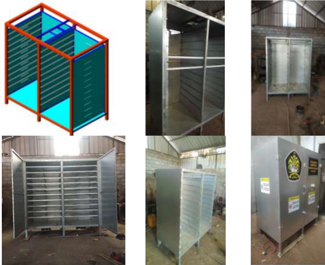
Fig. 3:-Designed salted fish drying oven.
