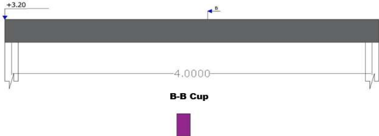
Figure 3:- Beam on two supports with a section of 15 \times 30 cm.
