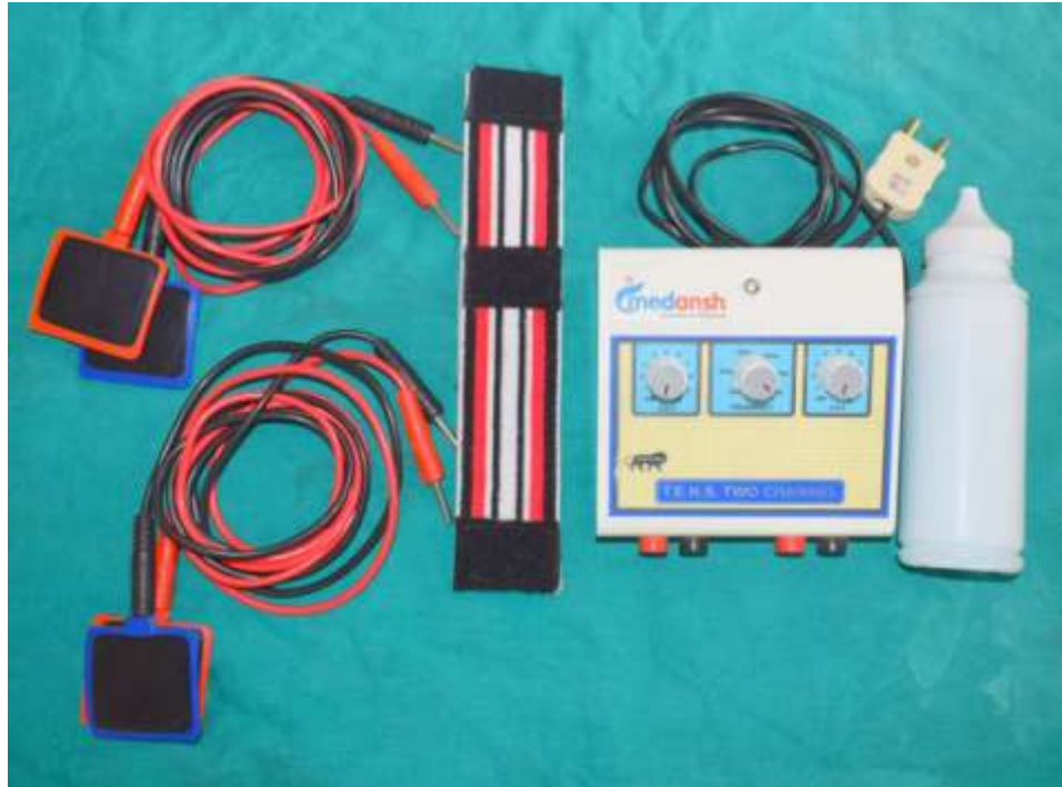
Figure 1:- Apparatus for TENS - Electrode pads with leads, Velcro strap, TENS device and Conductive gel.
