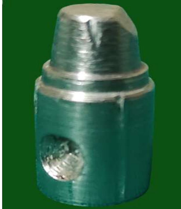
Fig No. I: Stainless-steel metal die (ANSI/ADA specifications).
