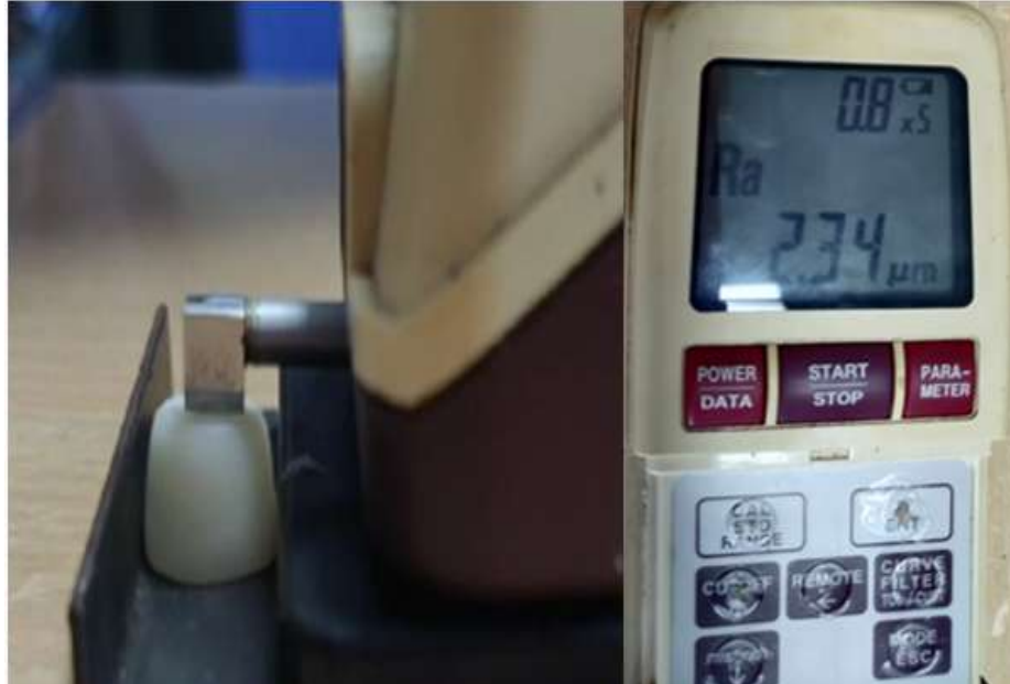
Fig No. V: Surface Roughness measured using Profilometer.
