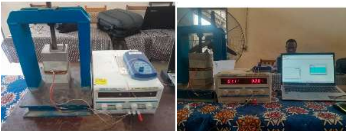
Figure 1:- Thermal characterization of CEB by the asymmetric hot plane method.
