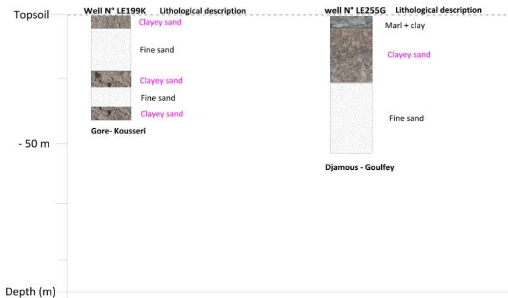
Fig. 10. A geological profile (with layers thickness) for borehole field of a GSHP system in Kousseri and Goulfey
