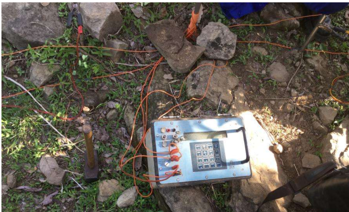
Fig.6. Vertical electrical sounding instrument SYSCAL PRO IRIS
