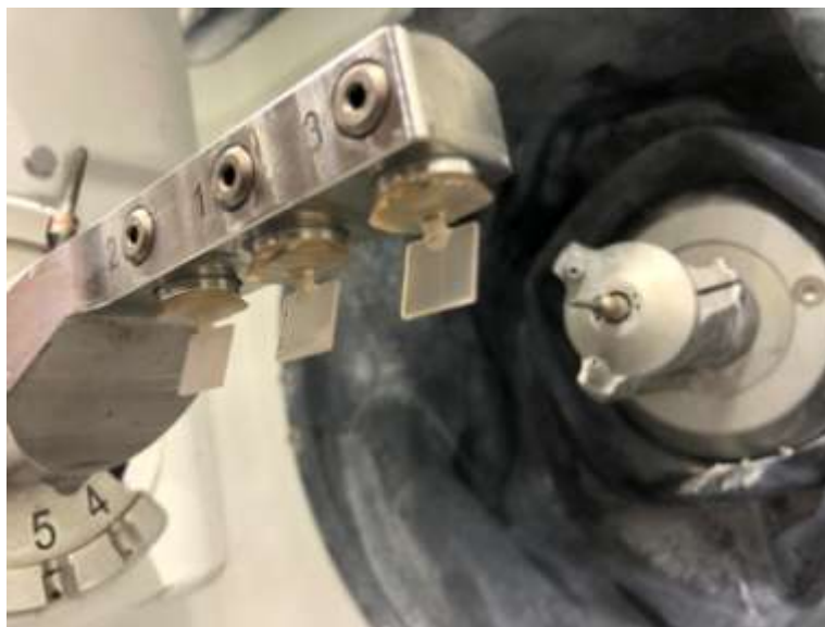
Fig 7:- Milling of LDS samples.
