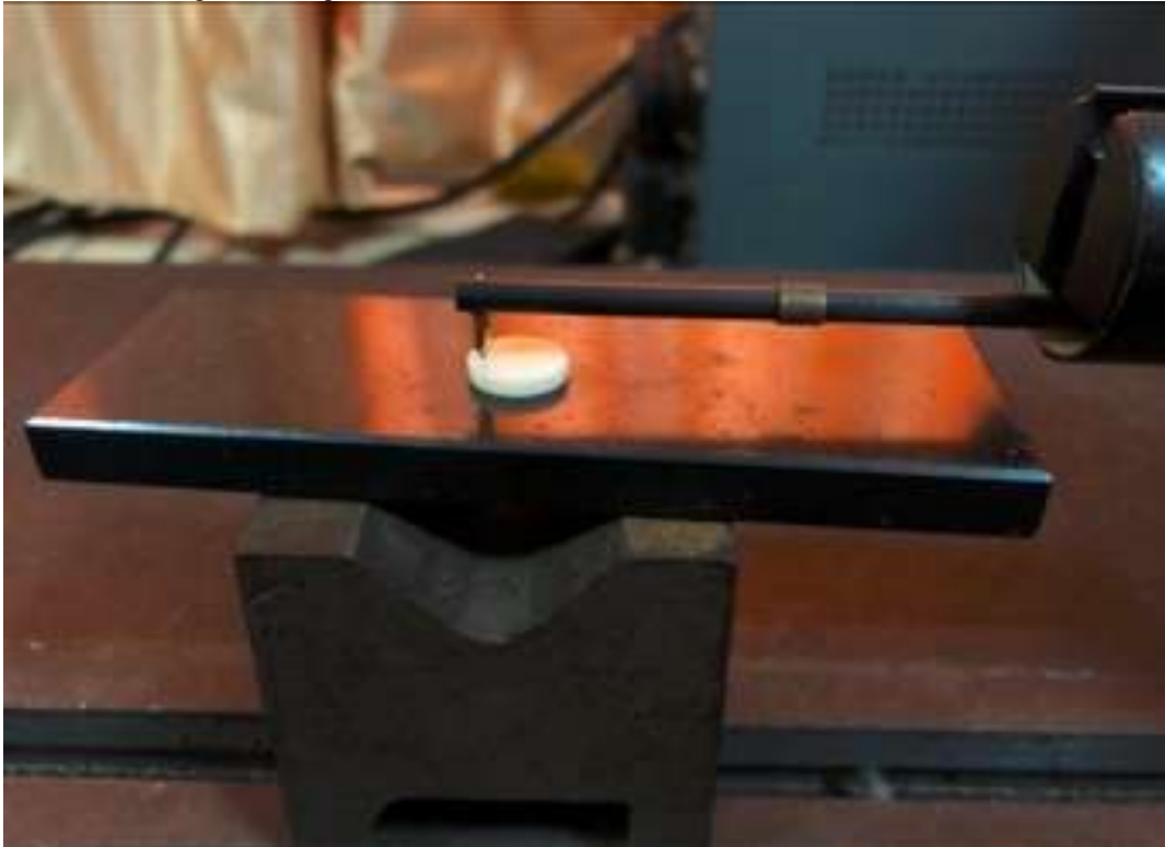
Fig 12:- Checking for surface roughness baseline values using profilometer (Mitutoyo Surface Profilometer SDA 350).
