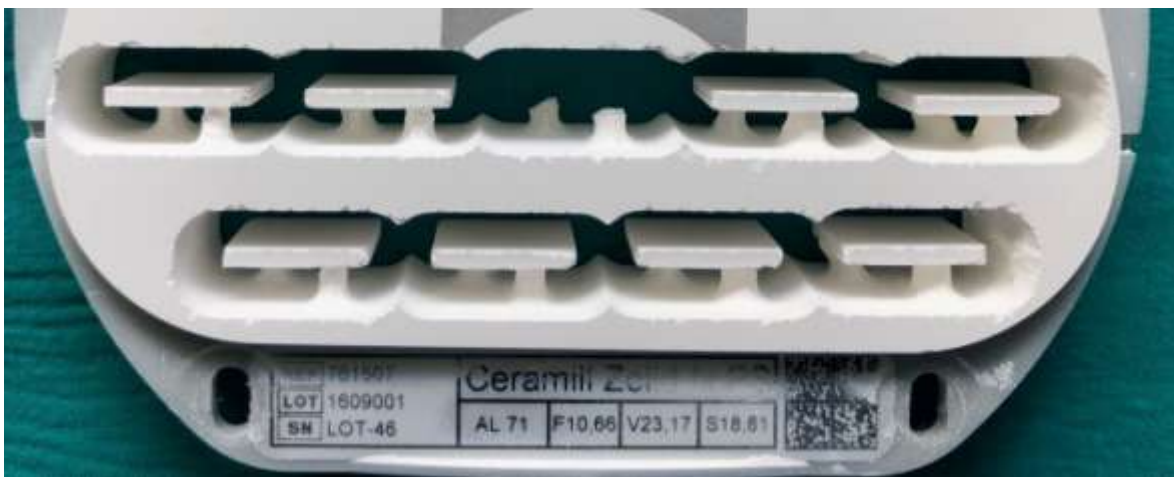
Fig 3:- Computer assisted milling of ZrSH samples:
