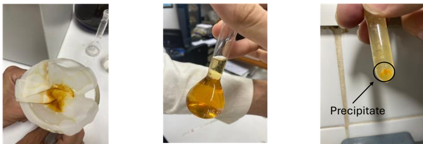
Figure 2:- IB solution before \text{FeSO}_4 and \text{H}_2\text{O}_2 addition (a), after addition (b), the release of \text{O}_2 (c), after filtration to collect the \text{Fe}(\text{OH})_3\downarrow (d), solution after filtration (e), and after centrifugation at 13,000 RPM/5 min. (f).
