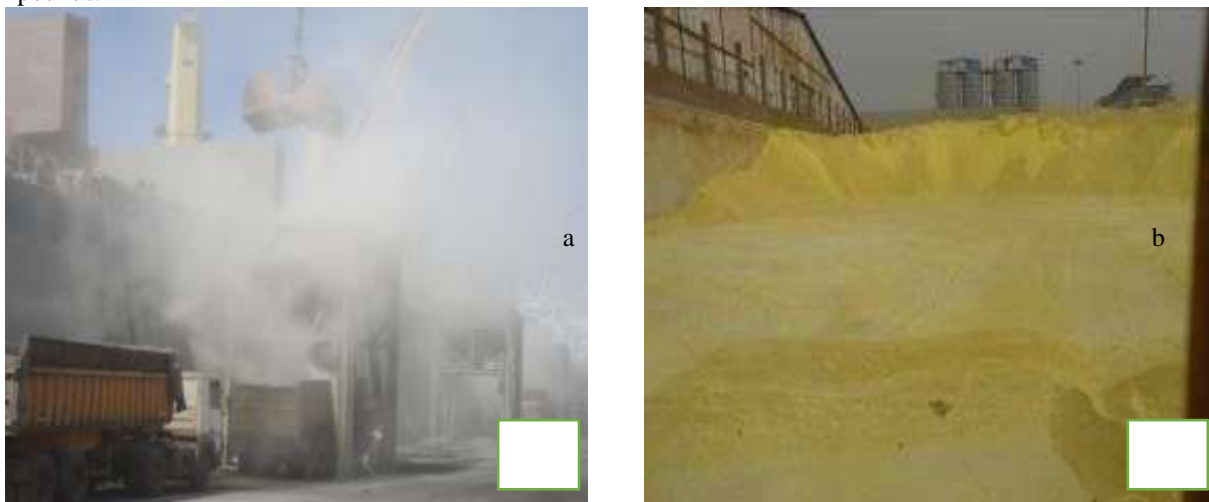
Plate 4:- Dust Emission During Clinker Unloading (a) and Sulfur Exposure in the Open at the Sulfur Yard (b). Photographer: Akiyo, 2019
