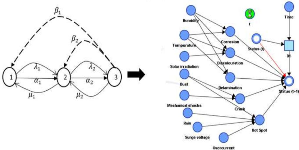
**Figure 1:-**Transition graph from the Markov model to the dynamic Bayesian model of the PV modules degradation
