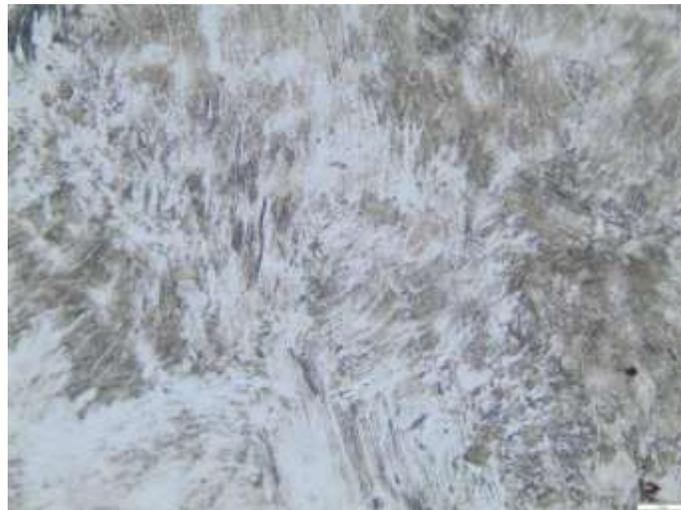
**Fig 1:-** Microstructure of Ti-48Al-2Cr-2Nb (Alloy 1)[200X].
