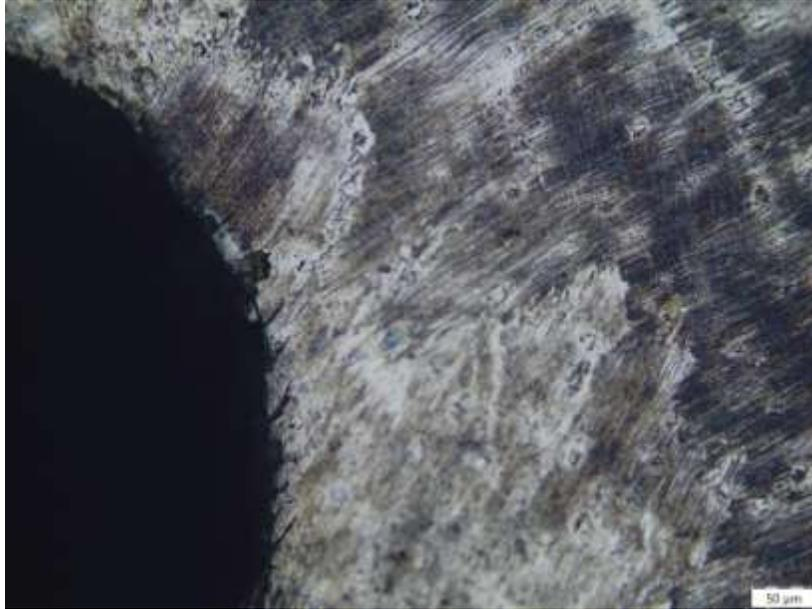
**Fig 8:-** Experiment 27 (8 A, 3 kW, 12  $\mu$ s pulse-on, 3  $\mu$ s pulse-off, 180 rpm): Oxidation films and prominent nodular deposits along the edges.
