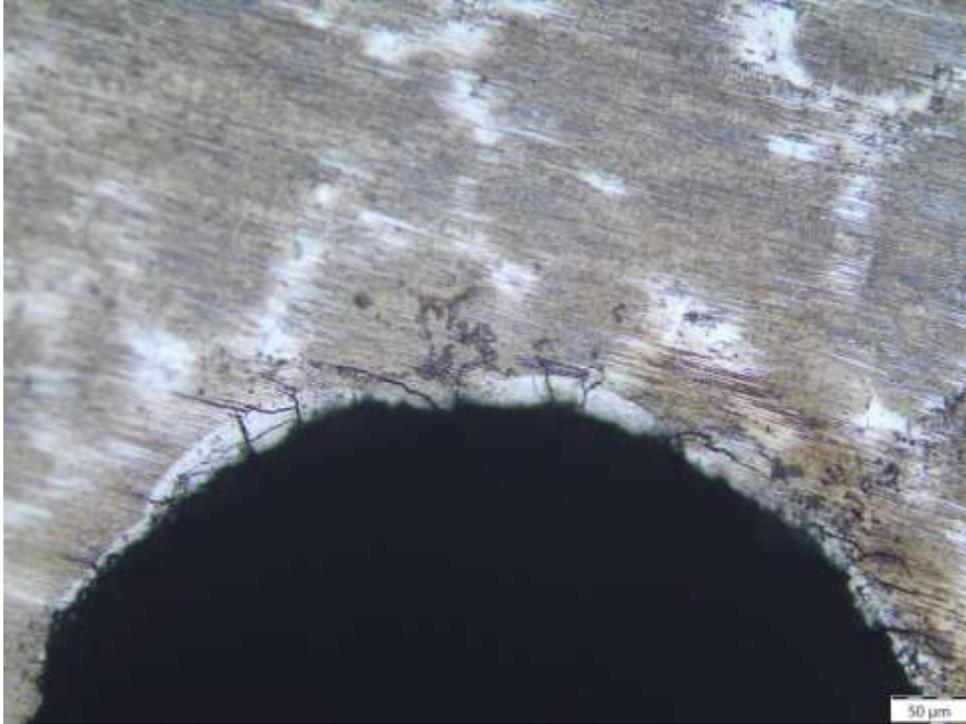
**Fig 3:-** Experiment 2 (4 A, 2 kW, 9 μs pulse-on, 6 μs pulse-off, 60 rpm): Thicker recast layer with minor micro-cracks near the edge. Some nodular deposits observed.
