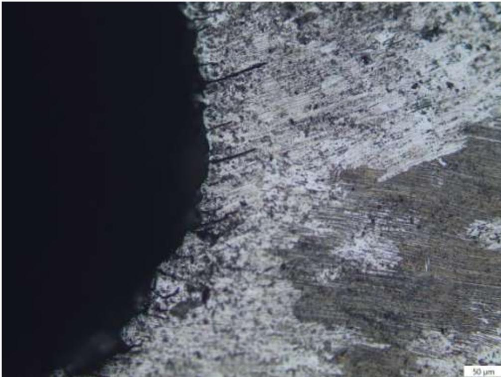
**Fig 5:-** Experiment 9 (6 A, 3 kW, 12  $\mu\text{s}$  pulse-on, 3  $\mu\text{s}$  pulse-off, 60 rpm): Significant nodular deposition, Oxidation evident.
