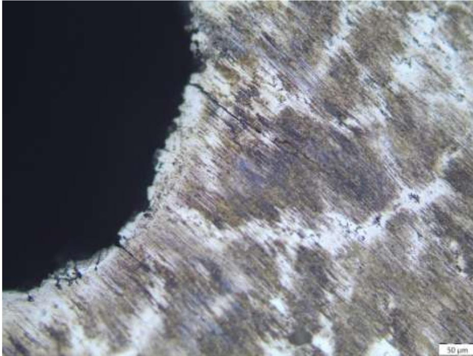
**Fig 2:-** Experiment 1 (4 A, 1 kW, 6  $\mu$ s pulse-on, 9  $\mu$ s pulse-off, 60 rpm): Minimal recast layer and negligible micro-cracks. Smooth boundaries due to the low discharge energy and adequate cooling time.
