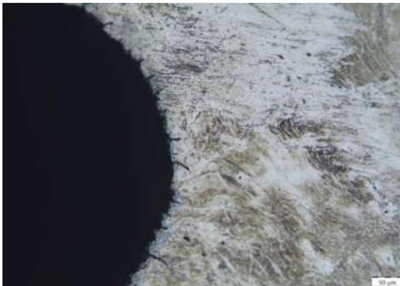
**Fig 7:-** Experiment 23 (6 A, 2 kW, 9 μs pulse-on, 6 μs pulse-off, 180 rpm): Micro-cracking observed. Small nodular deposits observed, with smooth boundary edges.
