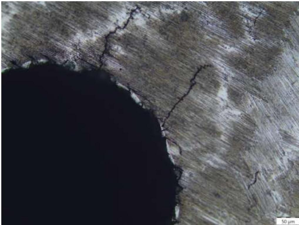
**Fig 4:-** Experiment 3(4 A, 3 kW, 12 μs pulse-on, 3 μs pulse-off, 60 rpm): Visible recast layer with more pronounced micro-cracks. Nodular deposits more frequent, and surface oxidation starts to appear.
