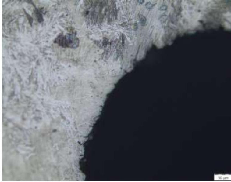
**Fig 6:-** Experiment 16 (8 A, 1 kW, 6 μs pulse-on, 6 μs pulse-off, 120 rpm): No visible micro-cracks.
