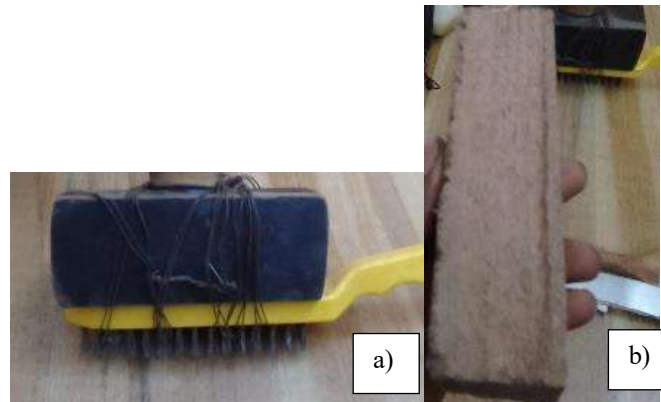
Figure 1:- Wear test of a CEB sample (a= wire brush and b= brushed surface of the sample).
