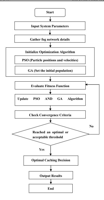
Figure 1: Proposed Flowchart for Fog caching using a NIOT
