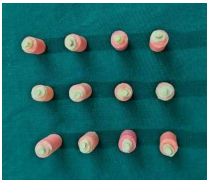
Figure 1:- Placement Of Rmgic And Equia Forte Into 3x3 Mm Cylindrical Mold.
