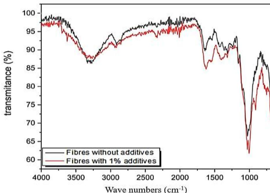
Figure 5:-ATR-FTIR spectra of coconut palm fibers, with and without starch added as an additive.
