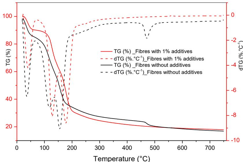
**Figure 4;**-Thermogravimetric analysis (TGA) and derivative thermogravimetry (dTG) curves as a function of temperature for coconut palm fibers, with and without starch added as an additive.
