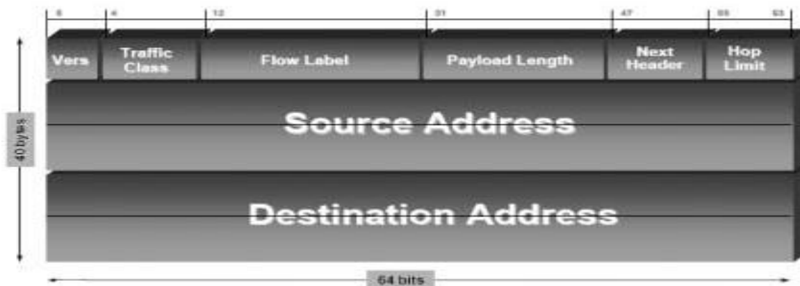
Figure no ( 4 ) Ipv6 base header
