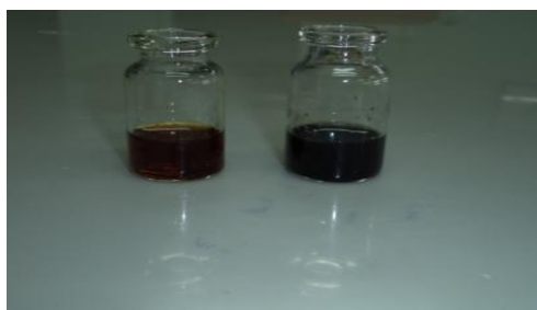
Figure 1. Qualitative test Tannins Using \text{FeCl}_3 Determination of Content of Total Tannins
