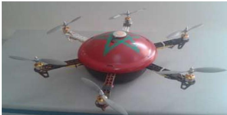
**Figure 1:-** A picture of the developed hexarotor(SMART\ENSEM).
