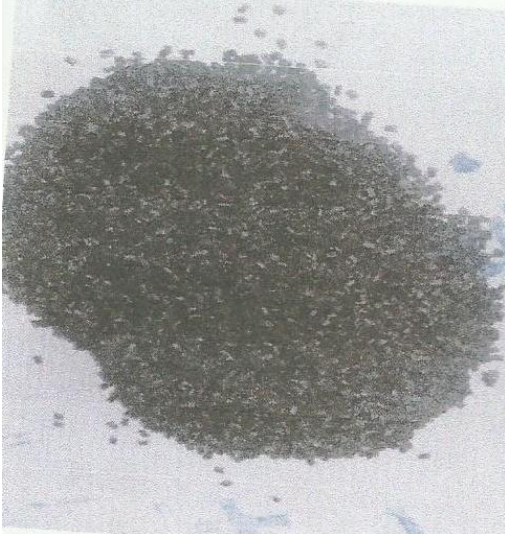
Fig. 3.3 shows samples of pellets obtained from the black films reclaimed
