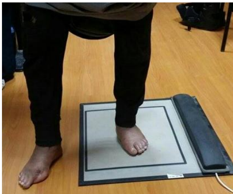
Fig. 5 Planter pressure assessment using plat form
