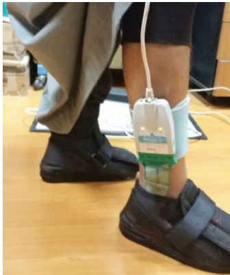
Fig. 4 Planter pressure assessment using in-shoe pressure measurement system
