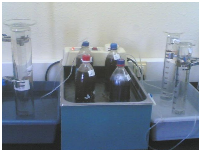
Figure 2:- The photograph of the experimental set up of biogas production and collection.
