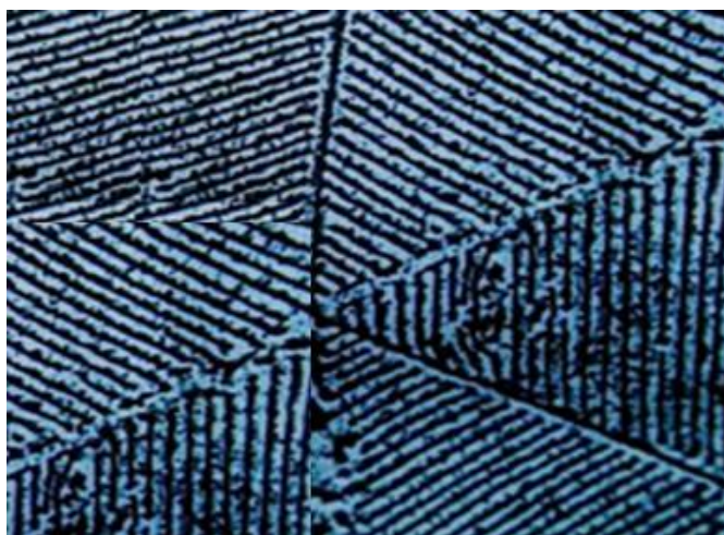
Fig.1:- Microstructure of pure Al metal (1500 x)
