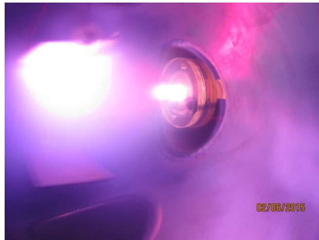
Figure 6:- Image of plasma from plasma gun in the presence of background plasma.
