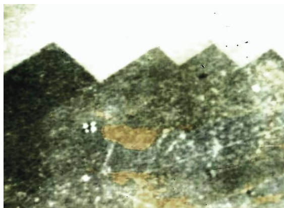
Fig. 2:- Microstructure of pure Bi metal (1500 x).
